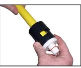
**8b** Chamfer end of pipe using Continental's double ended ID chamfering tool.
