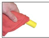
Chamfer end of pipe Sa using Continental's ID chamfering tool with ID gauge.
