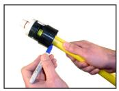
10 If using ID chamfer tool with gauge, check for proper chamfer by inserting pipe on gauge up to the o ring. With proper chamfer, o ring will begin to enter pipe.
